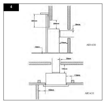
6.6 The void into which the appliance is fitted must be ventilated to prevent a build up of heat. If the void is sealed then it will be necessary to fit vents at both low and high levels of approximately 50cm<sup>2</sup>. These vents should take cold air from the room and return warm air back into the room.
